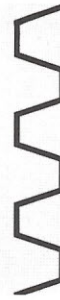
3 Universal stitch For firmer knits and wovens as well as felt, leather etc.
