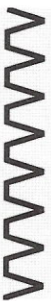
7 Vari-overlock Specially for fine synthetic and silk jerseys, Helanca and fine cotton and wool jerseys
